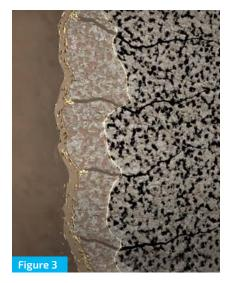
The result is a nearly impenetrable barrier against fluid and pressure invasion, which lifts off easily once differential pressure is released.
