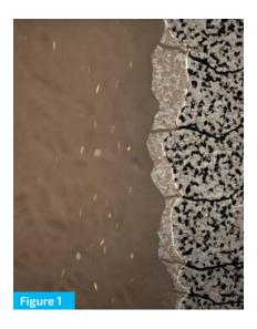
Initially, the FLC® Wellbore Shielding® particles are free-floating in the drilling fluid.
