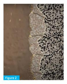
As differential pressure increases, the shielding particles work with mud solids to form a protective layer on the face of the formation.
