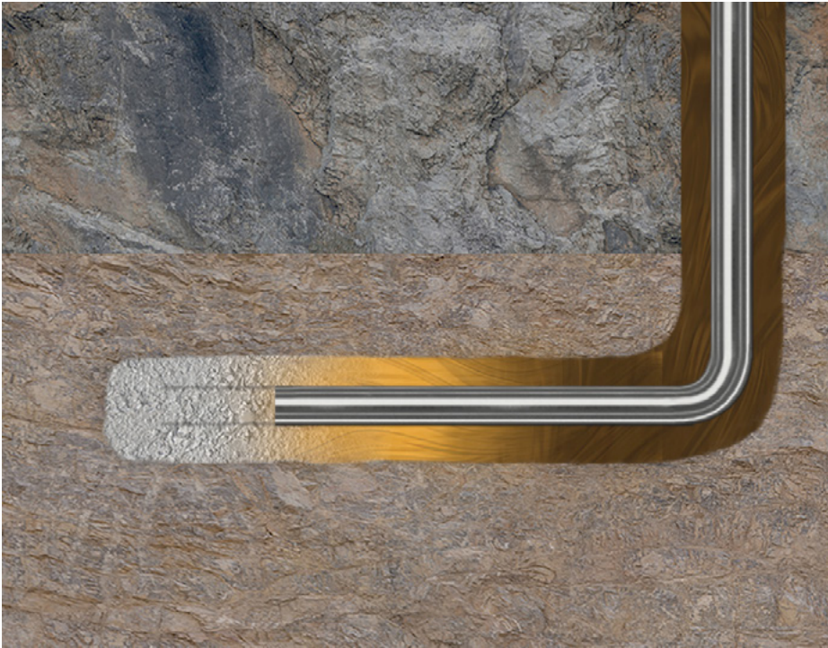
Figure 2. Spacer intermixing schematic (Source: Baker Hughes Co. and Impact Fluid Solutions LP)
