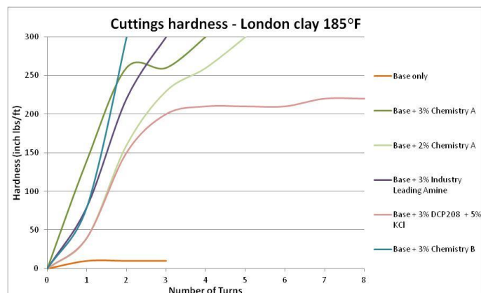
Figure 6. Hardness data on London shale of the two candidate materials (Chemistry A and B) versus two benchmarks KCl/poly(ethylene glycol) butyl ether (DCP 208) and an industry leading amine.
